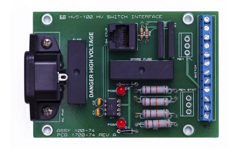
The HVS-100 HV Interface provides an update to older RF motorized switches that require 120/240VAC control and status. The HVS-100 converts the high voltage to a low voltage DC interface which is directly compatible with all BDI SWP-200/300 series RF switch controllers and remote control. This controller is completely solid state using solid state relays for high voltage control thus isolating high voltage AC away from low level control inputs.
